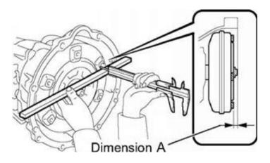
A. "Measure Dimension A: While holding the torque converter in place against the transmission, use a straightedge to measure the distance between the bell housing mating surface and the torque converter mounting pads. (Typical A-727 torque converter depth = 19/32", ±0.050".)
