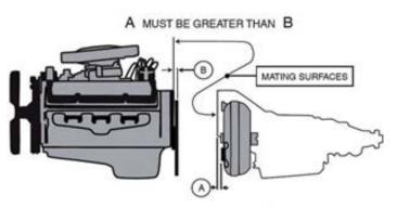
C. Verify that Dimension A is greater than Dimension B. If it is not, the torque converter is not fully seated. Pull it off slightly, then, while rotating it, push it back on. Continue to do this until you feel the torque converter move inward and make the proper engagement. Then repeat and compare Dimensions A and B. Do not proceed further until the torque converter is fully seated.
