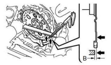
**B.** Measure Dimension B: On the engine, measure the distance between the engine block mating surface and the torque converter mating pads (the raised surfaces on the flexplate at each torque converter fastener hole).
