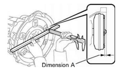
A. Measure Dimension A: While holding the torque converter in place against the transmission, use a straightedge to measure the distance between the bell housing mating surface and the torque converter mounting pads.
