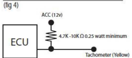
Setup the Tachometer to run 2 pulses per rev when connecting it to the engines' ECU.
