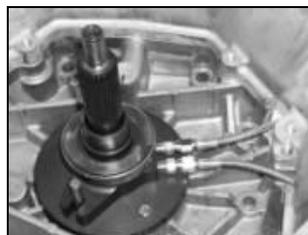
Adapting to your factory master cylinder is achieved by installing the proper quick connect adapter fitting in the master cylinder, shown in the following pictures:
