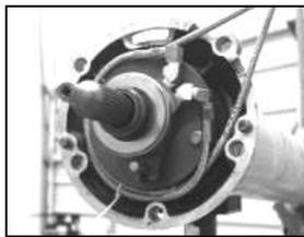
Adapting to your factory master cylinder is achieved by removing the roll pin and factory fitting from the master cylinder, and installing the provided adapter as show in the following picture:
