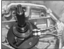
Adapting to your factory master cylinder is achieved by installing the quick connect adapter fitting in the master cylinder, shown in the following picture:
