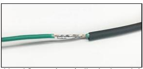
Soldered Connection w/ adhesive heat shrink
