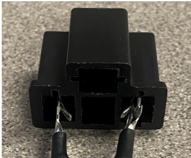
Example of completed adapter harness
