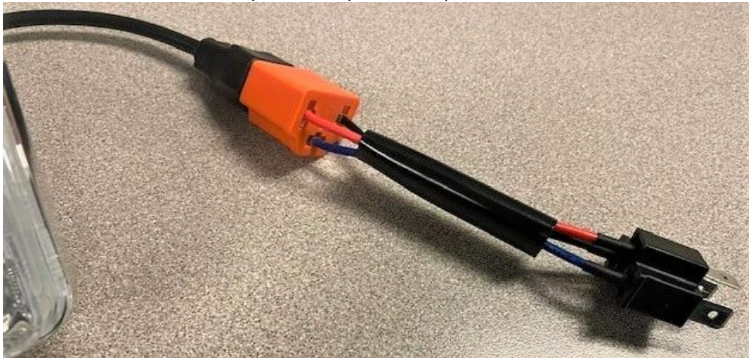
Example of completed adapter harness
