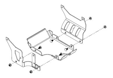
2. Bolt the shield assembly onto oil pan using the M8 x 16 Flange Head Bolts, leaving them finger tight.
