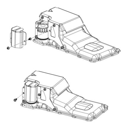
NOTE: Starting with the bolt, torque fasteners to 18 ft./lbs
