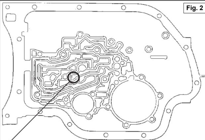
The 1988 and later TH-400 has a checkball in this location and must use Shift Improver Kit (#20261). If you have no checkball in this location, this kit (#20260) is the correct one.
