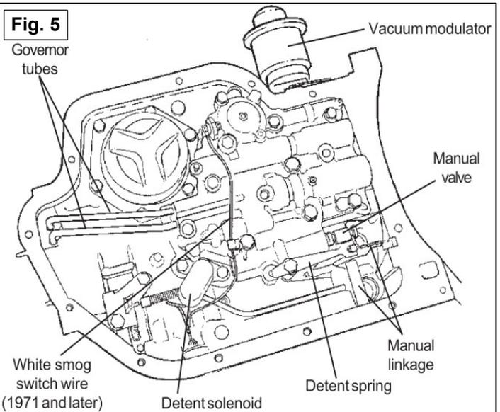
4. There are (3) 1/4-20 and (8) 5/16-18 (10 some early models) bolts holding the valve body. Remove all but one valve body bolt and disconnect the switch wire if present. Hold the valve body in place and remove the last bolt. Lower the valve body while at the same time pulling straight down on the governor tubes (See Fig. 6). Place the valve body in the oil pan to avoid contamination.
