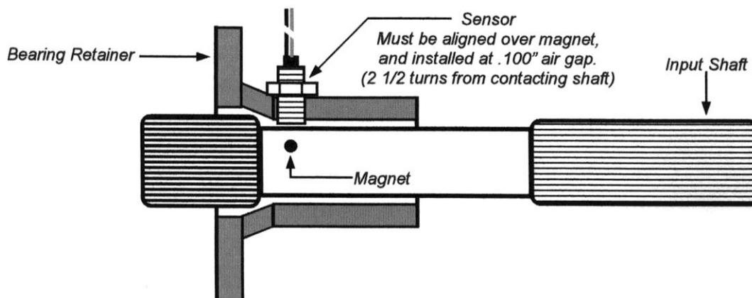
**Important!!** The supplied magnet will be marked on one end with yellow ink. Epoxy the magnet inside the input shaft with the yellow side facing upward. If your input shaft has a magnet pre-installed from the manufacture and you are not sure if the polarity of the magnet is correct you should contact RacePak at (949) 580-6898 to obtain more detailed directions on preparing the input shaft.
