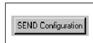
When finished sending the message "**Device Programmed Successfully**" should be displayed at the bottom of the progress box. If you receive an error message, turn power to the system off and then back on and repeat the send configuration process. If problems persist, check the troubleshooting section in your manual and then contact RacePak.
