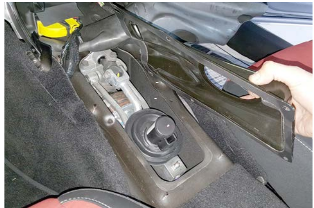
24. Remove the tunnel cover from the vehicle.
