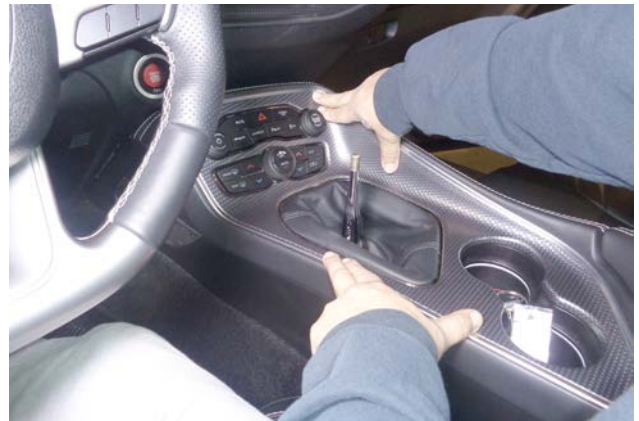
70. Snap the console bezel into the console.
