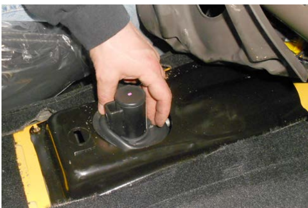
23. Push the edges of the shifter seal down and in to separate it from the tunnel cover.
