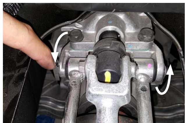
26. Rotate the locking tabs on the 2 shifter yoke pins clockwise until they face rearward, then remove the pins.
