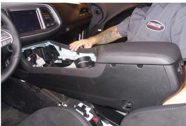
18. Move both front seats fully rearward, then carefully remove the center console from the vehicle.
