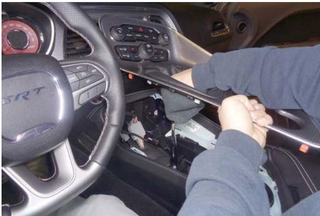
68. Move the console bezel into the vehicle, and carefully slide the boot opening down over the top of the shifter stick.
