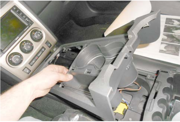
45. Snap the console cover into the center console.
