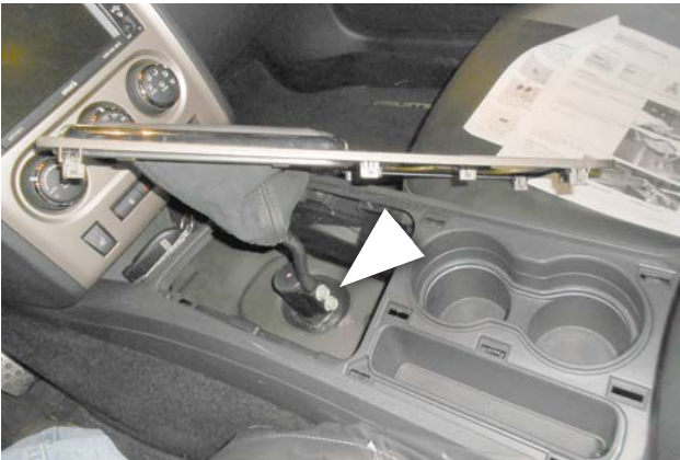
46. Hold the assembled trim bezel, boot, and stick above the console cover, and insert the stick in the slot on the rear of the shifter. Install the 2 OEM screws with thread-locking fluid, then tighten them to 20 lb-ft torque.
