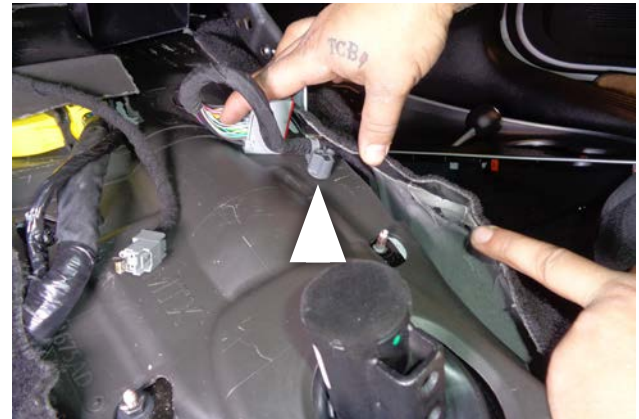
20. Detach the harness clamp from the button at the front right of the dust boot.
