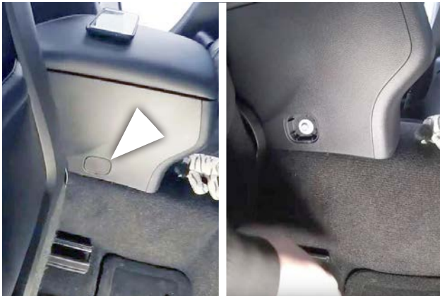
17. Move both front seats fully forward. At the bottom rear on each side of the console, remove the square trim cover and the screw beneath it (2 screws total).
