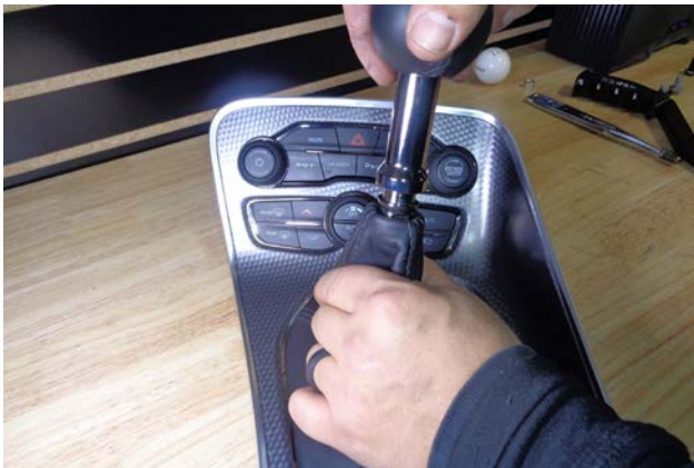
67. Carefully separate the elastic boot opening from the bottom of the shifter handle.
