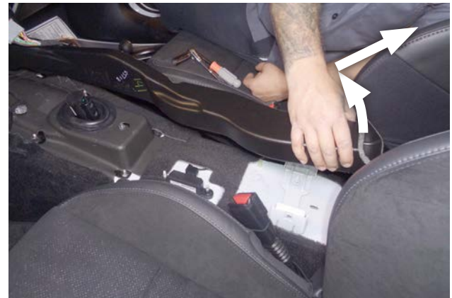
19. Lift the rear of the vent duct up sharply to release it. Then move the duct rearward to disengage its front end, and remove it from the vehicle.
