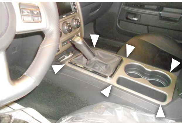
47. Snap the trim bezel back into the console cover.
