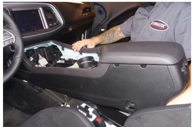
50. Carefully return the center console to the vehicle and place it in its final location. Be sure that the rear of the vent duct mates correctly with the opening at the rear of the console.
