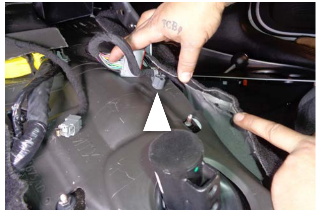
48. Push the harness clamp onto its button on the dust boot.
