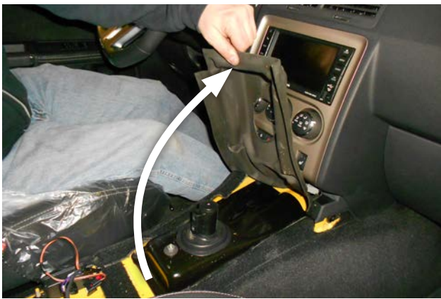
21. Fold the dust boot up and forward to access the tunnel cover fasteners.
