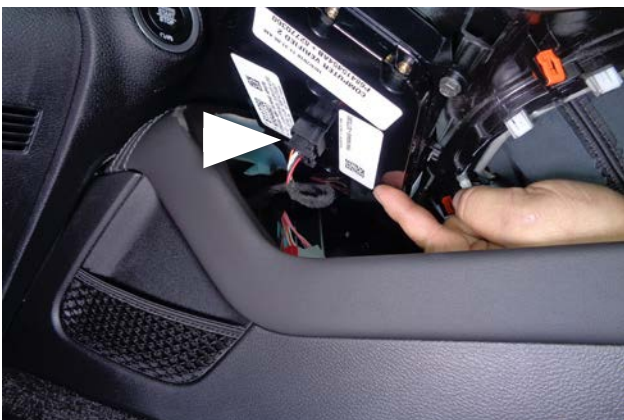
69. Reconnect the electrical wiring to the back of the control panel.
