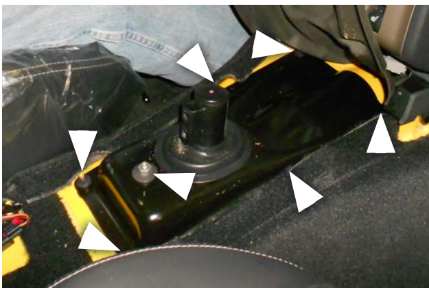
22. Remove all 7 nuts from the tunnel cover (1 to the rear of the shifter seal, and 6 along the sides).
