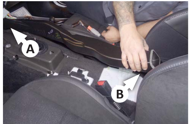
49. Insert the front of the vent duct into its opening (A) under the control panel, and snap it into place at the rear (B).
