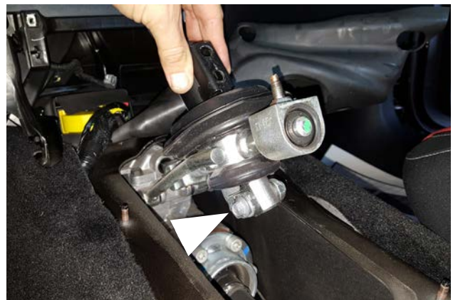
25. Remove the screw connecting the dog-bone link to the shifter.
