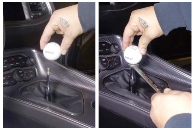
71. Thread the lock nut (5) fully down the stick (wrench flats down), followed by the shifter knob (4) . Then align the knob's shift pattern as desired, and tighten the jam nut.
