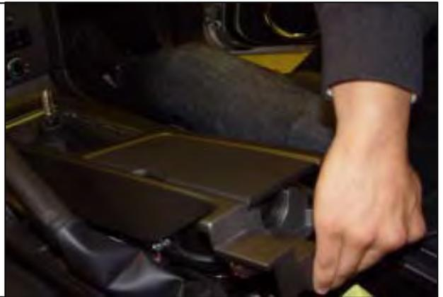
3. Disconnect the traction control/hazard light/trunk release and any other (cup holder lighting, etc.) wiring harness connectors that prevent removal of this center console trim plate. Then remove the console trim plate.
