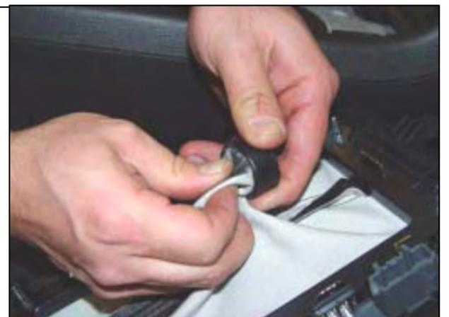
37. The factory shifter boot will need to be opened up in order slide it over the reverse lockout. Start by cutting loose enough threads so that the boot will slide over the lockout with a snug fit.
