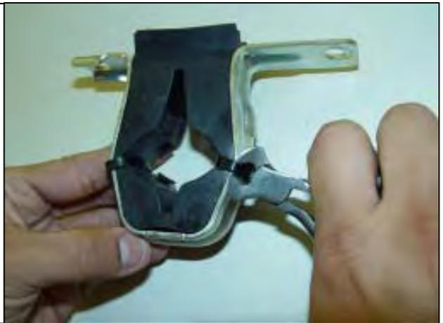
12. Pry off the lower bushing cup off of the shifter bottom pivot, being careful not to damage the soft plastic as this part will be re-used.
