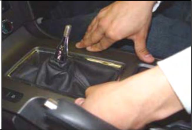
43. Screw the jam nut down onto the upper stick threads.
