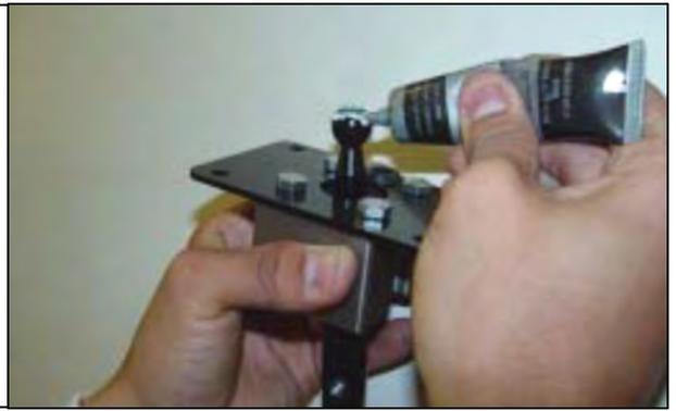
14. Place the plastic bushing cup (removed in step 12) onto a hard surface and snap the lower pivot ball of the Hurst shifter into the bushing cup.
