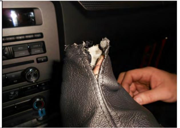
38. Invert the shift boot and slide it over the reverse lockout.
