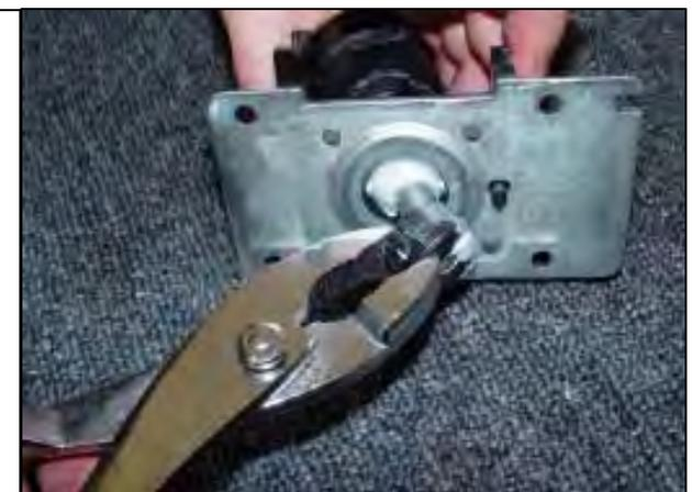
13. Grease the lower pivot ball of the Hurst shifter.
