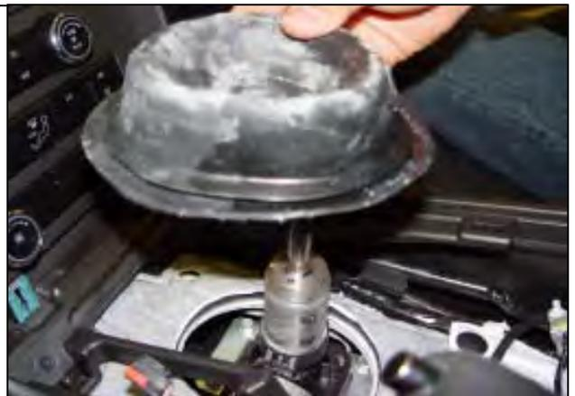
5. Remove the three (3) accessible screws of the four (4) screws holding the shifter to the shifter linkage housing.
