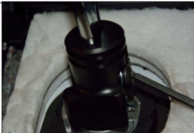
28. Install the extension spring to the Reverse Lockout Collar with the supplied Spring Retaining Screw.
