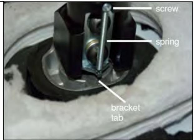
30. Add grease to the Lockout Collar where it rides against the guide nut.
