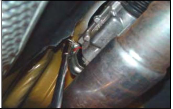
22. Insert the Trigger Rod into the Reverse Lockout Collar.
