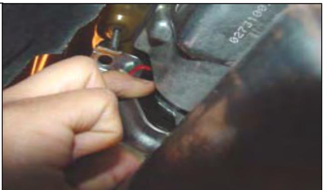
21. Push the rear bushing assembly onto the mounting studs and tighten the mounting nuts to secure the shifter assembly to the tunnel.
