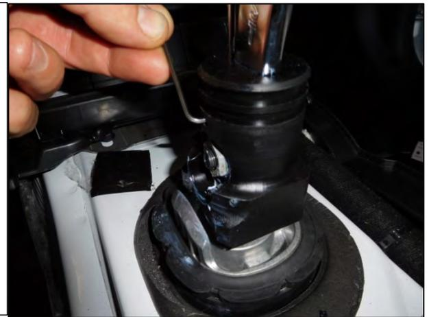
32. To prevent premature wear to the Reverse Lockout Collar, apply grease to the shifter reverse block and lock-out collar where the two will contact during shifts to 1st / 2nd gear.
