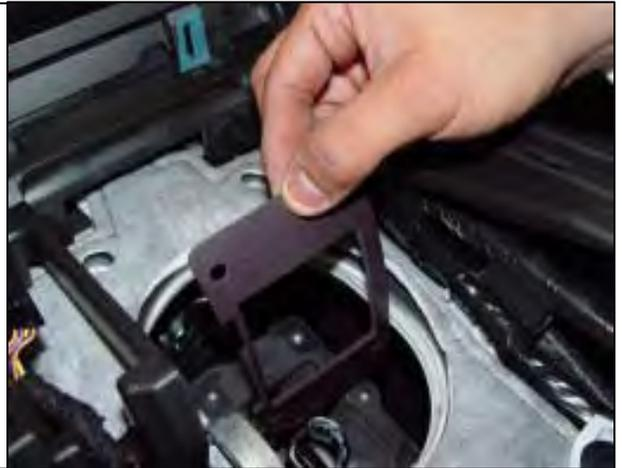
16. Place the Hurst Shifter on top of the foam gasket and shifter housing base and tighten the three (3) accessible screws.
