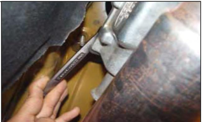
20. Push the rear bushing assembly onto the rear of the shifter base assembly.
