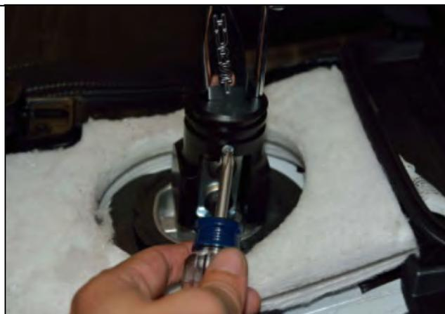
29. Insert the other end of the spring onto the Spring Bracket tab.
