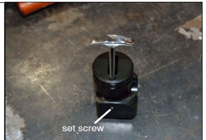
25. Thread one of the supplied nylon set screws into the upper hole on the left side of the block. Screw it in until it just begins to protrude into the slotted center opening.
