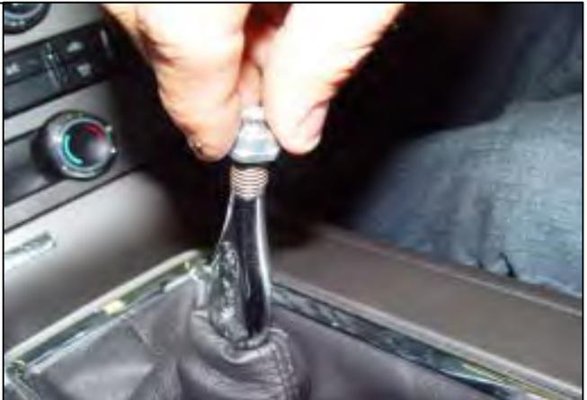
44. Install the shift knob onto the stick. Align the logo on the shift knob accordingly and tighten the jam nut up against the knob. A few drops of Loctite will help prevent the knob from loosening.
