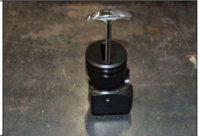
23. Insert the cotter pin through the hole in the Trigger Rod. Bend each leg of the cotter pin 90 degrees and cut excess material. The photo to the right is a bottom view of the assembly. Please note the orientation of the cotter pin and the approx. length of the legs.
