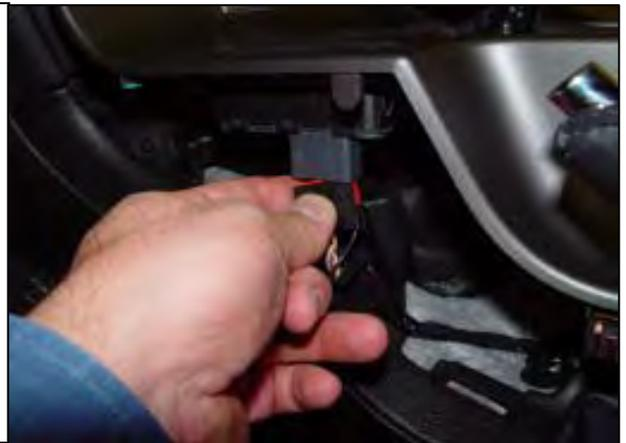
4. Remove the rubber boot that seals the shifter to the tunnel.
