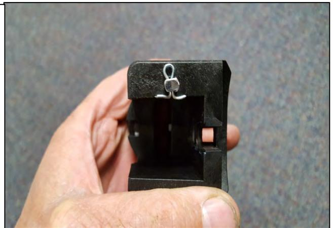
24. Align the Trigger Rod so that the top is perpendicular to the opening in the Reverse Lockout Collar. While maintaining the alignment, pull up on the Trigger Rod so that it is at its highest position within the Reverse Lockout Collar and secure it in position with the steel set screw.
