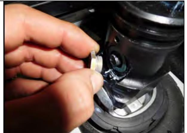
31. Use an allen wrench to adjust the nylon set screw that was installed in step 25. Adjust as necessary to reduce side to side play and get the block to slide up and down freely. Once it's adjusted properly insert a second nylon set screw and tighten against the first to lock in place.
