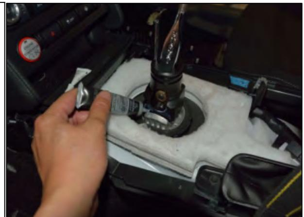
33. The reverse lockout must be adjusted so that the shifter can smoothly be shifted into first gear while not being able to shift into reverse without pulling up on the T handle. Adjustment can be made by sliding the lockout and securing it into position by tightening down the 4 bolts.
