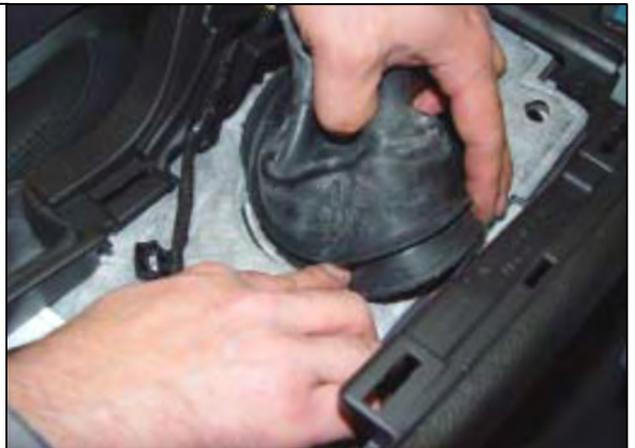
36. Carefully peel the leather shift boot away and off of the plastic boot collar. The plastic collar will not be re-used.
