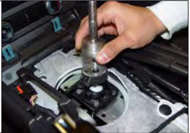
11. Trim the tie wraps from the rear bushing assembly, remove the rubber bushing from the bracket.
