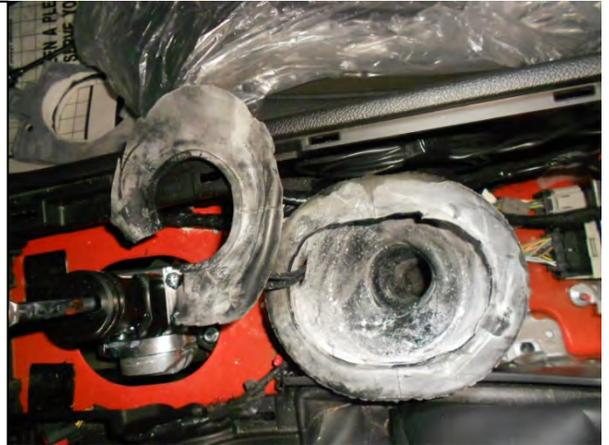
35. Work the rubber boot seam onto the shifter access-hole edge so that it fully seals the tunnel hole.
