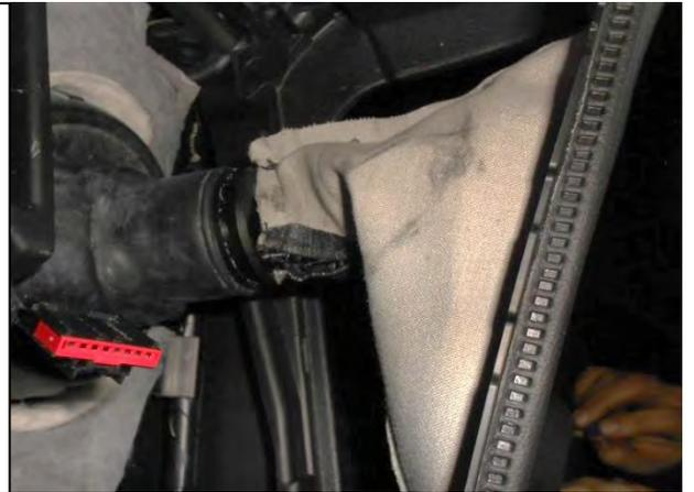
39. Although the zip tie installed in the next step should prevent any further unraveling to the sewn seam of the shift boot, you can place a small amount of super glue (not supplied) onto the stitching to keep it from unraveling.
