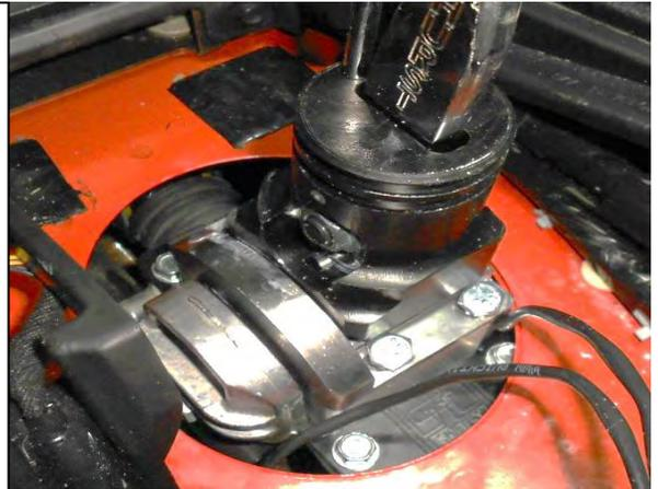
34. The bottom of the factory rubber boot will need to be trimmed in order to clear the Hurst shifter
