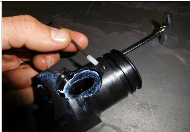
26. Install the Upper Chrome Stick and Spring Bracket. The 3/8" guide screw will be inserted and installed into the bottom hole of the stick along with a 3/8" lock washer and a 3/8" washer.
