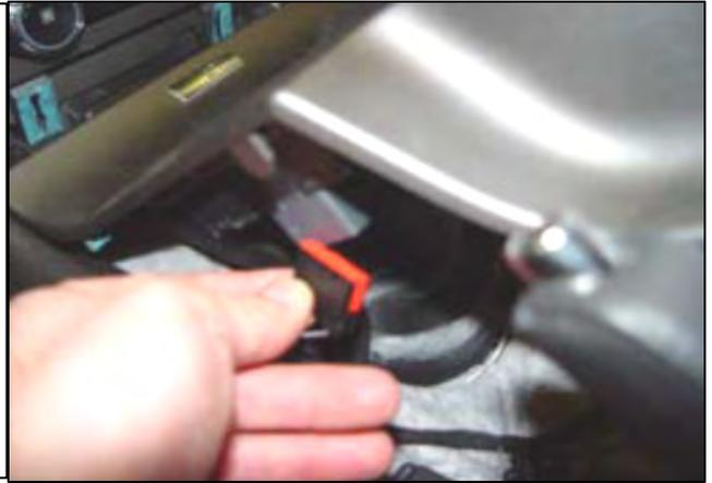
42. Snap the center console trim cover/cup holder unit back into place.
