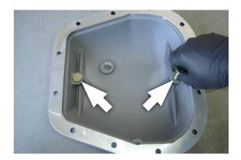
11. IF USING RTV SEALANT: Apply a continuous bead of gear oil-compatible RTV silicone sealant to the cover's flange. Run the sealant between the screw holes and the inside edge of the flange.
