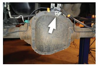
**NOTE:** On some vehicles, access to the cover may be made easier by loosening / removing surrounding parts (sway bar, brake line bracket, Panhard rod, etc.).
