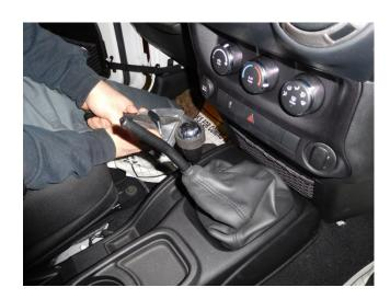
2) Grab the back of the center console by the cup holders and pull up to un-clip the console to remove.
