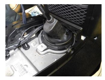
19) Reinstall the center console and press the factory knob onto the shifter and transfer case stick.
