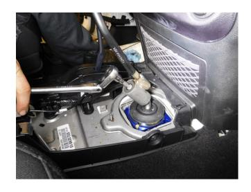
18) Reinstall the rubber boot over the factory shifter stick and secure it to the floor with the factory square flat nut.
