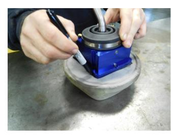
11) Carefully cut along the inside line marked out to allow the B&M shifter to fit securely.
