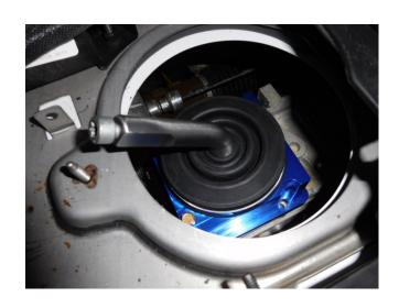
15) Reinstall the shifter donut from the interior side down over the shifter.
