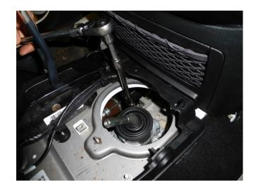
13) Wipe clean with a lint free towel or rag around the shifter base area and apply black rtv silicone sealer to the base.
