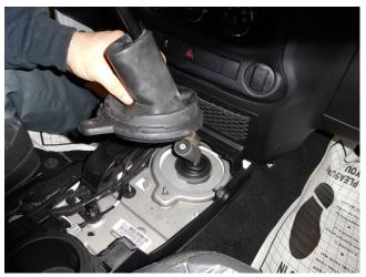
4) Use a ratchet and T45 torx socket to remove the bolt in the center of the shifter.
