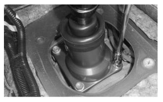
**16. Re-install the stock shifter screws,** and tighten to 13 ft-lbs torque.
