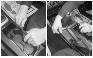
**4. Use a plastic trim removal tool** to separate the upper console panel from the console base.
