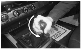
2. Remove the shift knob by unscrewing it from the shift lever.
