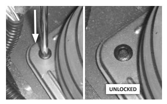
**8.** Unlock the 2 plastic push rivets at the front of the cover plate by depressing their center plungers slightly (about 1/16") with a punch or small Phillips head screwdriver.
