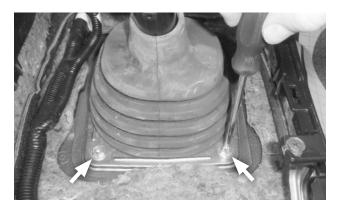
23. Re-install the 2 cover plate screws.
