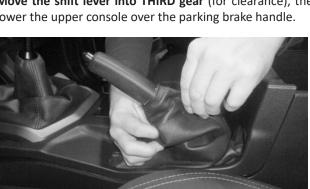
28. Work the leather boot down over the parking brake lever, working its elastic opening into the groove on the lever.
