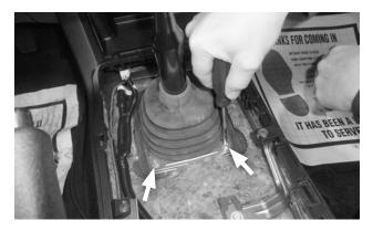
7. Remove the 2 screws at the rear of the cover plate assembly.
