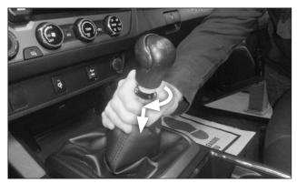
Detach the chrome trim ring from the shift knob by twisting it clockwise and pushing it downward.
