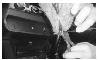
**26. Secure the boot to the lever** with the new cable tie, locating the buckle at the flat at the rear of the groove. Tighten the cable tie, and cut off the tail.
