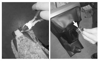
**24.** On the upper console panel, turn the leather boot insideout, cut the cable tie, and remove the chrome trim ring.
