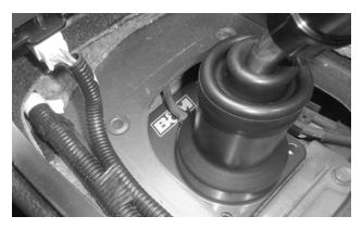
**15. Install the vent hose on the fitting** on the front of the shifter.
