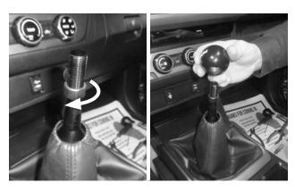
30. Run the jam nut all the way down the threads, then install the shift knob.
