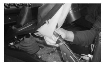
5. While lifting the console panel upward, turn the parking brake boot inside out, and work its elastic opening over the end of the parking brake lever.
