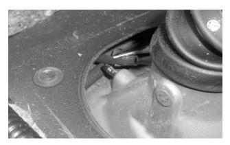
**10.** Carefully remove the rubber vent hose from the barb fitting on the front of the shifter housing.
