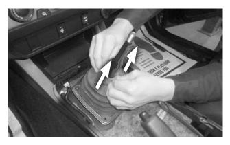
**9. Remove the cover plate,** working the rubber boot up over the shift lever, and set it aside.
