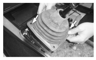
21. Lower the rest of the cover plate assembly over the shift lever, carefully working the boot's opening around the screw heads on the lever.
