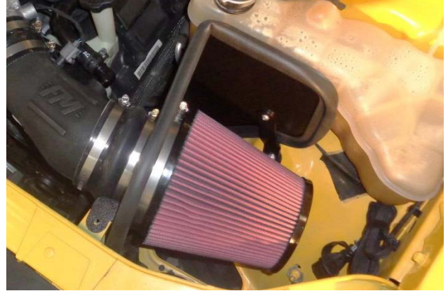
20. Install clamp (2) on air filter (1), install filter on filter adapter and tighten clamp.
