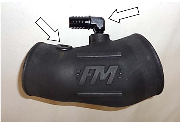
14. Install rubber grommet (17) in intake tube (14). Apply 2 wraps of nylon thread tape to threads of barbed elbow (18), and install elbow in tube.
