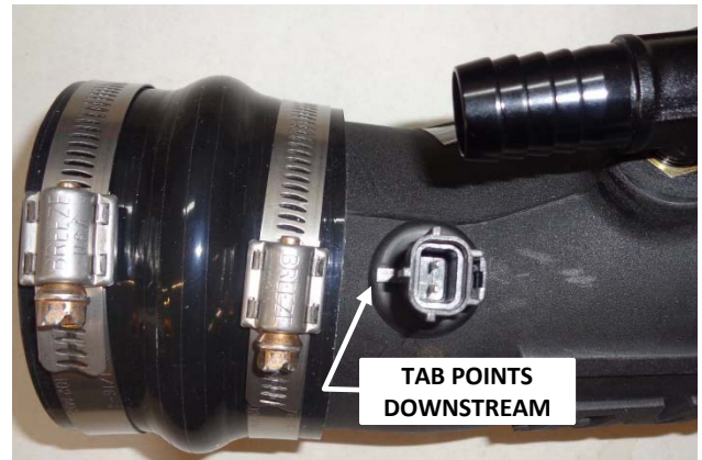
16. Carefully insert the inlet temperature sensor into the grommet, ensuring that the tab points downstream. (NOTE: Moistening the grommet with soapy water will ease insertion.)
