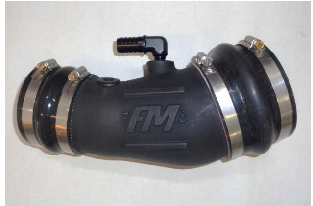
15. Install two small hose clamps (16) on small flex coupler (15), and install coupler on discharge end of intake tube. Install two large hose clamps (20) on large flex coupler (13), and install coupler on intake end of tube.
