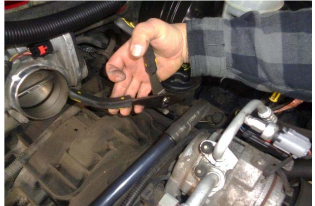
10. Disconnect the PCV hose from the base of the oil filler neck and remove the tube from the vehicle.
