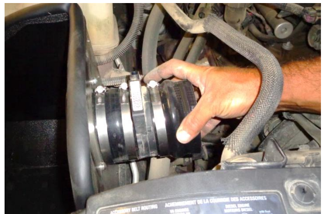
18. Slip 2 screw clamps (10) onto a flex coupler (11). Install the coupler on the MAF sensor, pushing it flush against the sensor. Tighten only the sensor clamp – leave the other clamp loose.
