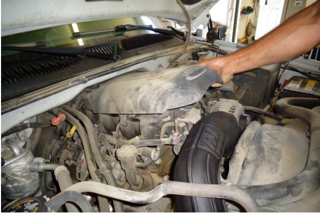
25. Install the engine appearance cover.
