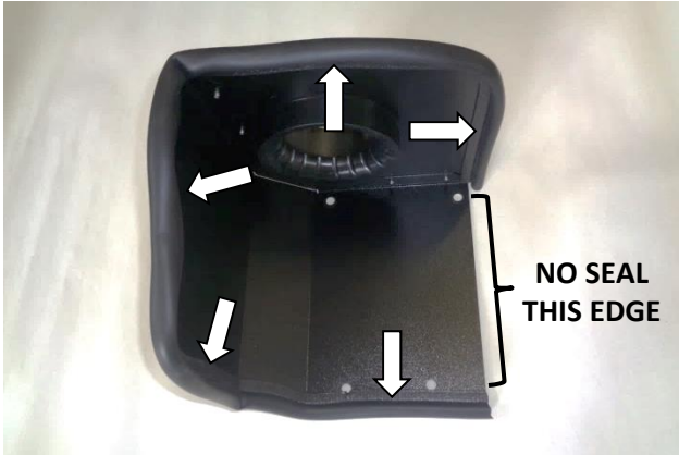
13. Attach the gasket (4) to the heat shield (5) along the edges shown. Starting at one end, press the seal fully onto the edge, gradually working around the heat shield. When you reach the end point, trim the gasket to fit using metal-cutting shears.
