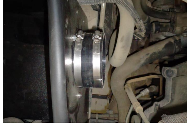
16. Slip 2 screw clamps (10) onto a straight coupler (9). Install the coupler on the filter adapter, pushing it flush against the heat shield. Tighten only the filter adapter clamp – leave the other clamp loose.
