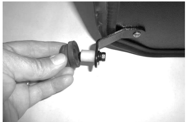
23. Attach nylon spacer (27) to bracket using \frac{1}{4} -20 \times 1 1/4" screw (24), lock washer (8) and flat washer (25) (against bracket), and nut (7) (against spacer). Install rubber bushing on spacer.
