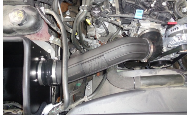
22. Install the intake tube in the vehicle.
