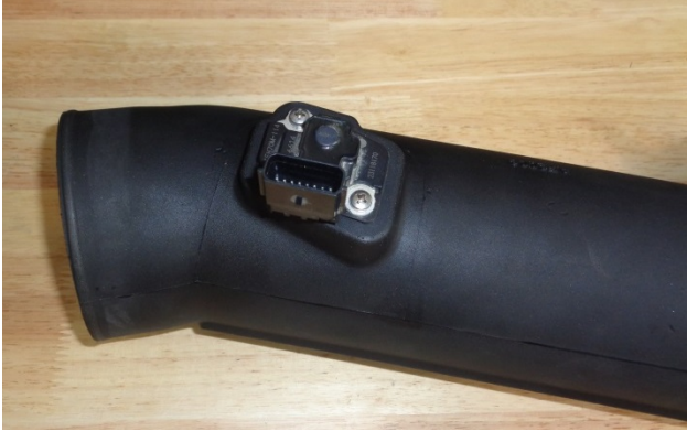
19. Install MAF sensor gasket (11) on the sensor, ensuring correct orientation. Then install sensor in intake tube, using M4 screws (12).
