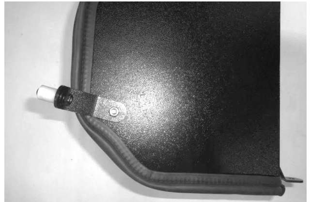
22. Attach bracket (27) to airbox using \frac{1}{4} -20 \times 5/8" screw (3) and flat washer (4) (against airbox), and nut (7) and lock washer (6) (against bracket). Leave bracket slightly loose until installation of airbox.
