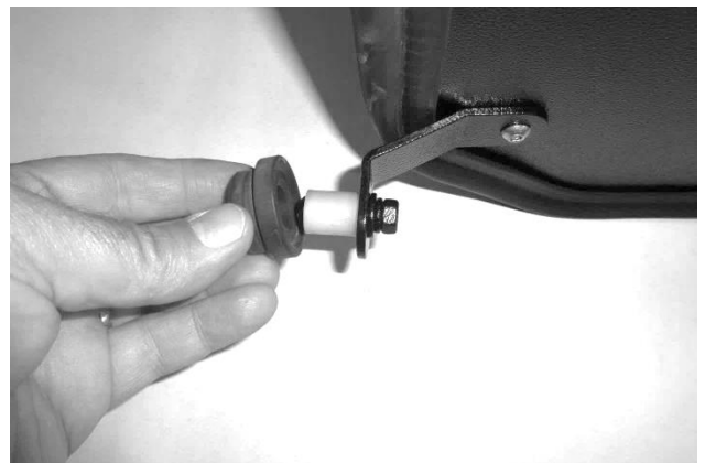
23. Attach nylon spacer (28) to bracket using \frac{1}{4} -20 \times 1 1/4" screw (26), lock washer (6) and flat washer (4) (against bracket), and nut (7) (against spacer). Install rubber bushing on spacer.
