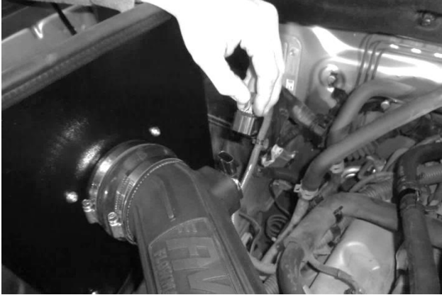
36. Reinstall the connector on the MAF sensor and verify that it is secure.
