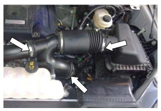
4. Loosen the screw clamps on the three ends of the air intake duct.
