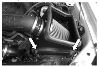
17. Secure the heat shield to the airbox with the two latches.
