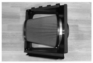
12. Slip screw clamp (2) onto air filter (1), then install the filter on the filter adapter and tighten the clamp. If desired, install pre-filter (17) over the cone element.
