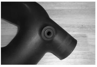
Install grommet (15) in intake tube (12).
