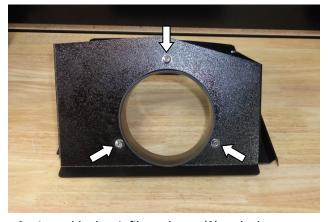
9. Assemble the air filter adapter (3) to the heat shield (4) using the M6 screws (9), lock washers (8) and flat washers (7).
