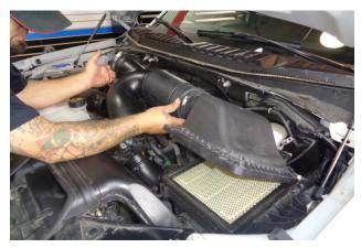
Separate the intake duct from the two turbocharger inlets, remove the assembled intake duct and airbox cover from the vehicle, and remove the stock air filter.
