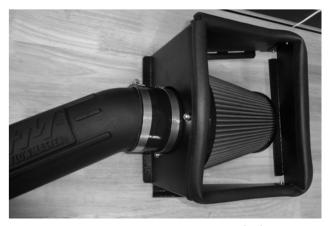
15. Slip the other two large screw clamps (10) onto the 4" straight coupler (11). Install the coupler onto the air filter adapter, pushing it flush against the heat shield, and tighten the clamp. Insert the intake tube in the coupler, and snug – do not tighten – the tube clamp at this time.
