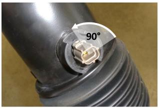
8. To remove the inlet air temperature sensor from the intake duct, lift its locking tab, rotate the sensor a quarter-turn counter-clockwise, then pull. Remove the o-ring from the sensor. CAUTION: The sensor is delicate! Handle it with care, and store it in a safe location until reinstallation.
