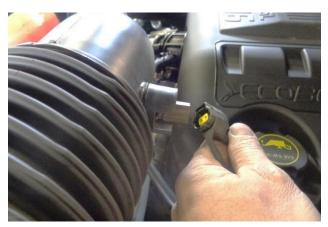
5. On the back of the intake duct, disconnect the inlet air temperature sensor plug.
