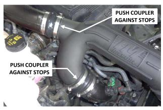
18. Push each coupler up against its stops on the turbo duct and tighten its turbo duct clamp.
