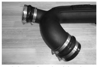
14. Slip the two small screw clamps (13) onto the 3" flex coupler (14). Slip two large screw clamps (10) onto the 4" flex coupler (16). Push each coupler onto the intake tube. Snug – do not tighten – only the tube clamps at this time. (Leave the other clamps loose.)
