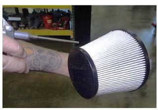
Blow off the outside of the filter. Blow across the filter surface (at about a 45° angle), not through the filter material. Hold the air nozzle about 6 inches away from the filter surface, always keep it moving, and point the air jet in to—not across—the pleats.
