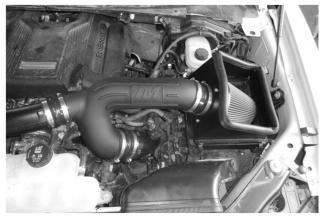
16. Insert the four tabs on the heat shield into the slots at the back of the airbox. Lower the tubeheat shield assembly, and connect the two couplers to their turbo ducts. Do not tighten the clamps at this time.
