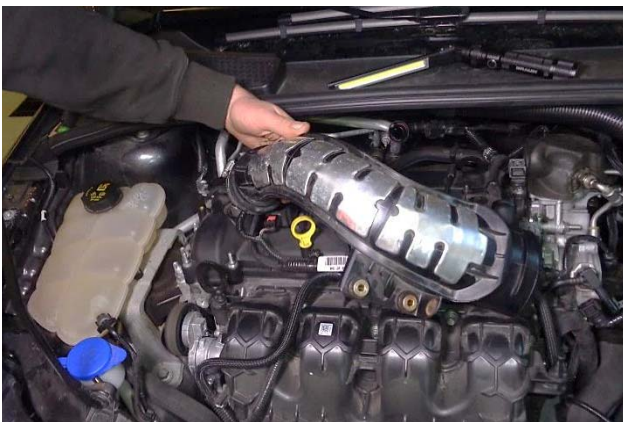
21. Separate the rear duct from the turbo inlet and remove it from the vehicle.
