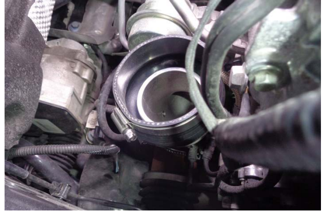
34. Install the small end of the coupler on the turbo inlet, push it flush against the raised lip, and tighten the clamp.
