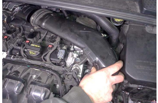
16. Separate the front duct from the rear duct and remove it from the vehicle.
