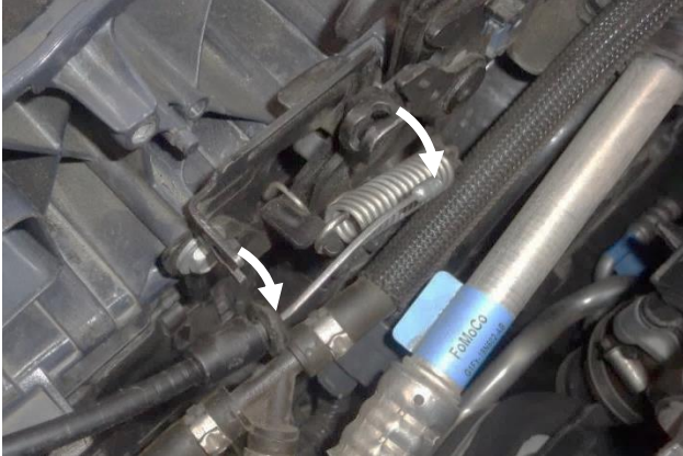
13. Remove the hood release cable end and grommet from the latch mechanism.
