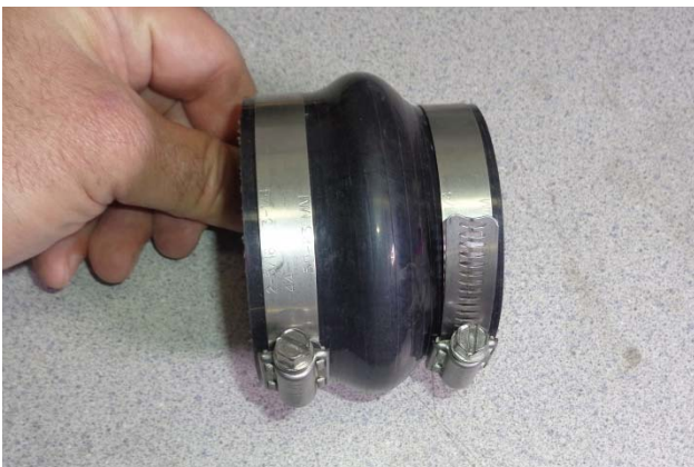
33. Install two small screw clamps (19) on the small reducing coupler (21). Do not tighten clamps at this time.
