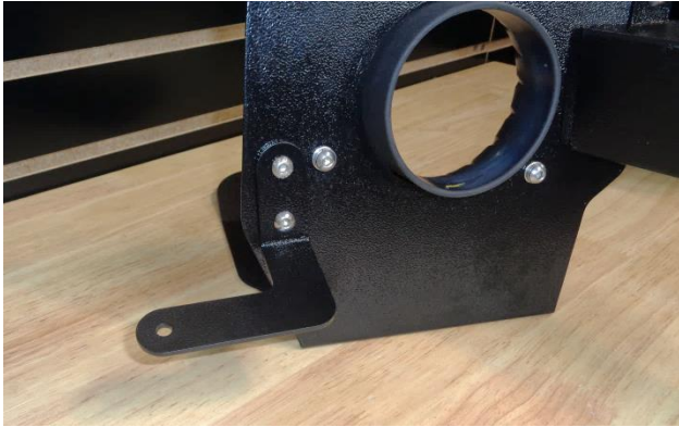
25. Attach bracket (26) to the heat shield using ¼-20 screws (25) (on the bracket side), and flat washers (11), lock washers (10) and nuts (9) (on the heat shield side).
