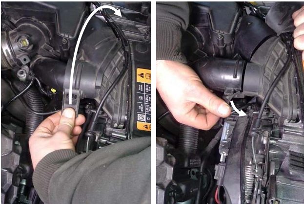
8. Release the two overlapping tabs to release the inlet air duct from the airbox.
