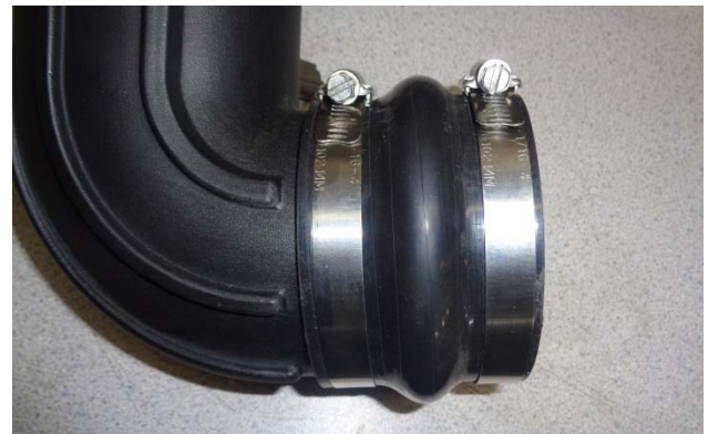
41. Install two large screw clamps (15) on the large flex coupler (16), and install the coupler on the end of the intake tube near the sharp elbow. Do not tighten clamps at this time.
