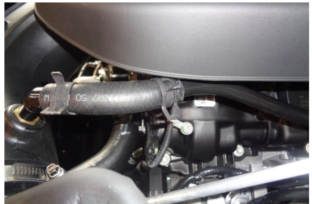
35. Verify there is no contact between the engine cover and the pinch clamp on the PCV tube. Adjust the pinch clamp if required.
