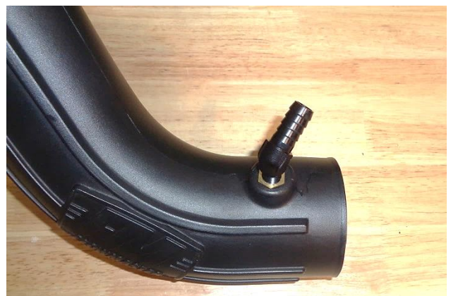
24. Apply 2 wraps of nylon thread tape to the threads of the barbed elbow (21), and install it in the intake tube (20).
