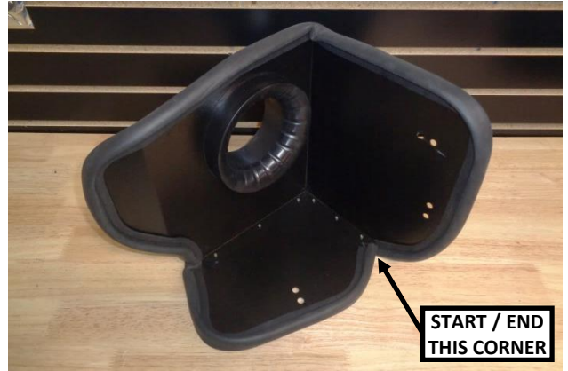
16. Attach the gasket (5) to the heat shield. Starting at the corner shown, firmly press the gasket onto the edge, gradually working around the heat shield. When you return to the starting corner, trim the gasket to fit using metal-cutting shears.
