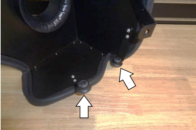
19. Push the two rubber grommets removed from the airbox at Step 12 into brackets (12) and (11) as shown.
