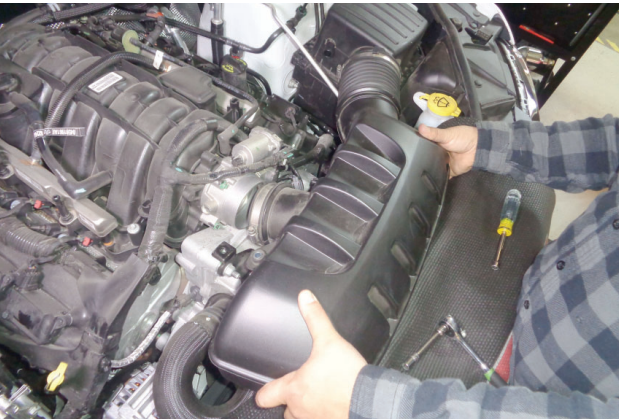
8. Remove resonator from engine compartment.
