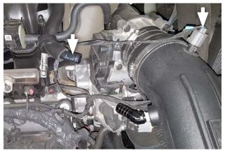
18. Reconnect the temp sensor wire to the sensor, and reinstall the wire holder on the crankcase vent line (removed Step 4).
