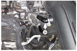
16. Apply thread tape to the **45° hose fitting (14),** and thread it into the intake tube.
