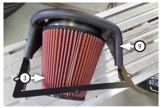
Push gasket (9) onto the edge of the heat shield as shown, cutting off the excess length with metal shears. Install the air filter (3) onto the adapter with the included clamp.
