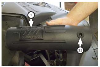
12. Install grommet (13) into intake tube (1).
