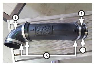
Place 2 hose clamps (8) on elbow coupler (5), and place hose clamps (7) and (8) onto reducer coupler (6). Fit the couplers onto the intake tube as shown.
