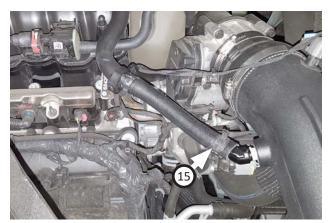
20. Place **pinch clamp (15)** onto the other end of the hose, push the hose onto the fitting, and move the clamp over the fitting to secure the hose.
