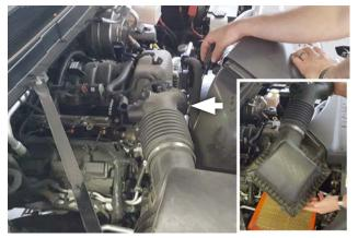
6. Loosen the clamp on the throttle body. Then remove the assembled airbox cover and intake duct from the vehicle as shown.
