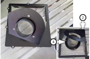
Assemble the air filter adapter (4) and heat shield
