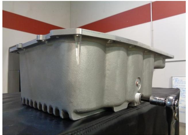
5. Inspect and wipe clean the stock oil pan gasket. If the gasket is in good condition, it can be re-used.
