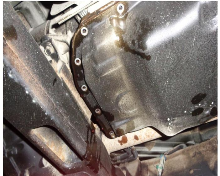
3. Remove the magnet from the stock oil pan and secure it on the B&M pan with the supplied hardware.
