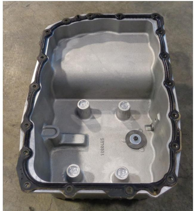
6. Clean the transmission mounting surface and install the B&M pan onto the transmission with the supplied M6 allen bolts and washers, qty. 18. Torque pan bolts to factory torque specs.
