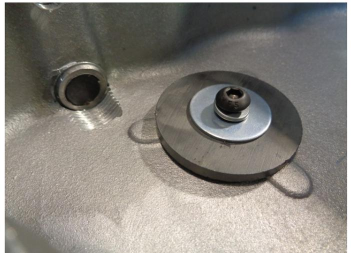
4. Install the 1/8 accessory pipe plug and then install the drain plug, be sure to use thread tape on the drain plug threads.
