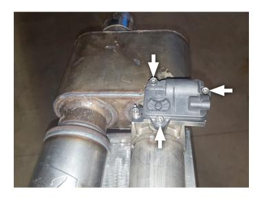
8. Install muffler into cut out section of factory exhaust then secure it using **clamps (x2) (9)**. Tighten them just enough to allow for adjustment.
