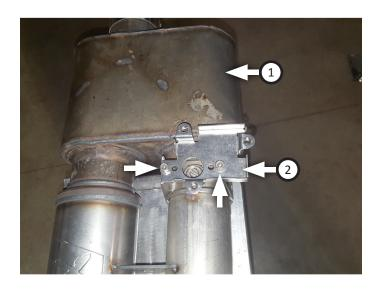
6. Place **valve spring (3)** onto groove in muffler outlet as shown.
