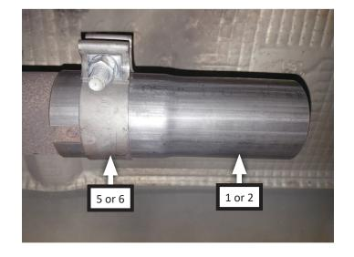
7. Place clamp (6) onto muffler (3) then connect it to adapter pipe, oriented as shown. Tighten clamp just enough to allow for later adjustment then place another clamp (6) onto muffler outlet.
