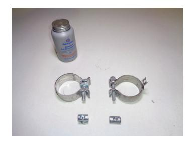
6. If your converter outlet is 2½": Place **clamp (5)** onto **adapter pipe (1)** then connect it to catalytic converter.
