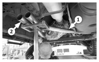
7. Attach left and right inlet pipes (2 and 1) to factory exhaust with the 2 stock gaskets, and 4 screws and springs, ensuring that both pipes are oriented properly.
