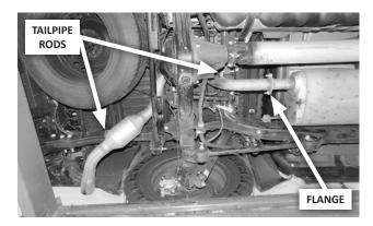
**2.** Remove 2 nuts at the tailpipe flange. Disengage tailpipe rods from rubber isolaters (2 places).
