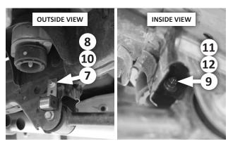
12. Install frame hanger (7) at the rearmost hole in the driver side lower control arm mount, using **bolt (8)** and **flat washer (10)** (against the hanger), and **fender washer (11)**, lock washer (12) and nut (9) inside the frame. Snug the fasteners slightly (to allow tailpipe installation, and final adjustment, later).
