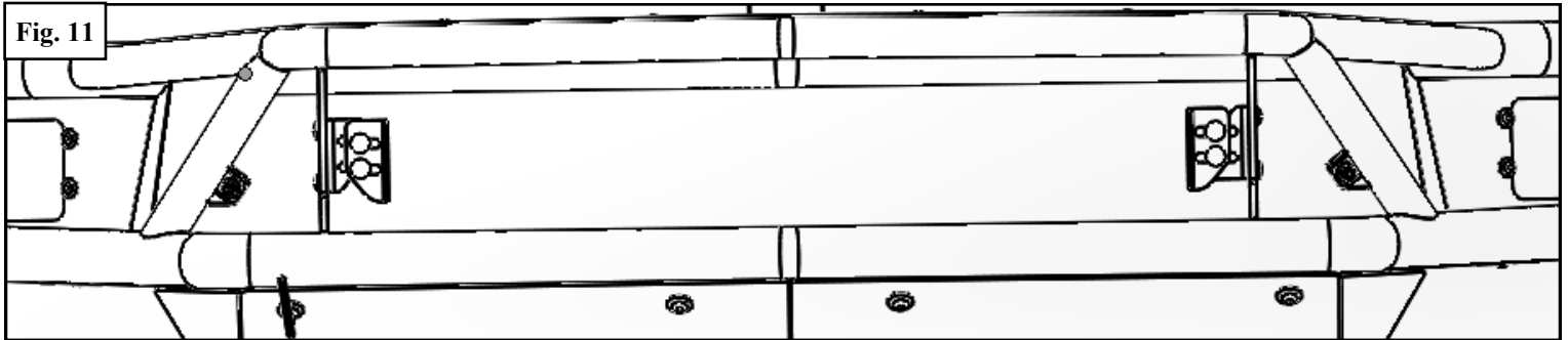
Figure 11 is an example showing the LED brackets adjusted in for the shortest light bar configuration.
