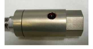
**3.** Carefully install sensor into load cell sensor port trying to minimize fluid loss during process.
