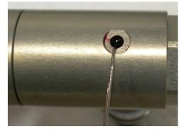
**5.** Re-insert bleed screw. It is normal for a slight amount of fluid to seep out while tightening the screw. Wipe load cell clean and install on vehicle.
