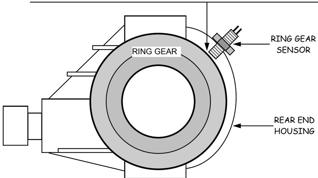
**IMPORTANT:** The jam nut on the sensor must be non-ferrous on either of these application.
