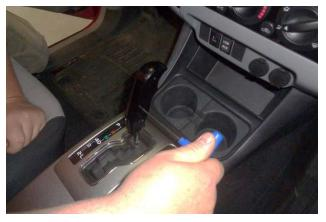
4. Properly align the shift handle by backing it up slightly, then tighten all four set screws.
