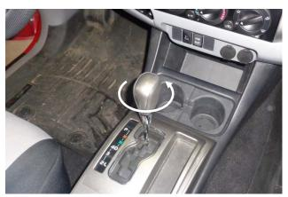
1. <u>Turn off your vehicle's ignition and set the</u> <u>parking brake</u>. Remove the stock shifter handle by rotating it counter-clockwise on the shifter stick.
