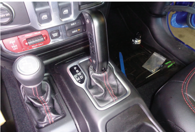
15. Clip boot cover into console cover and fit console cover back into place onto console.
