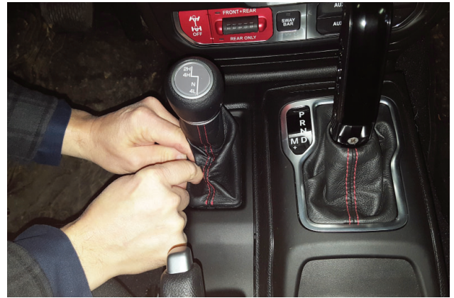
16. Unclip transfer case shifter boot from frame then pull it up to expose screw in its side.
