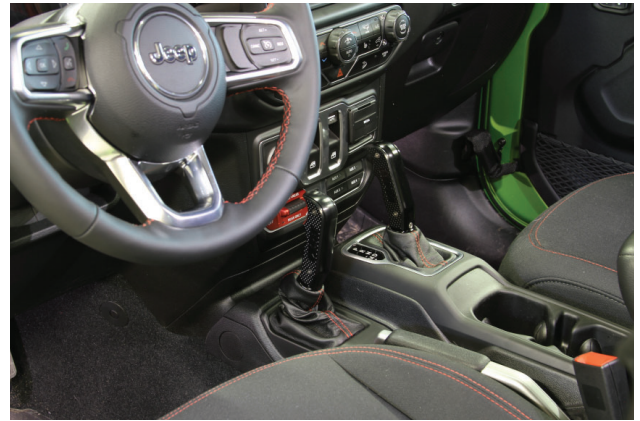
Congratulations, the installation of your B&M Magnum Grip AT Handle Set is now complete!
