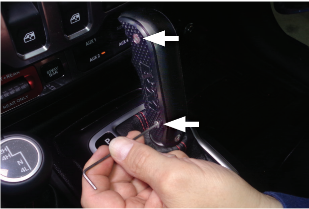
14. Reinstall screws and left shifter plate (removed step 11) onto shift handle body.
