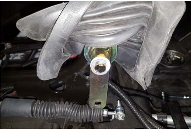
7. Lift rubber boot then remove and retain E-clip.
