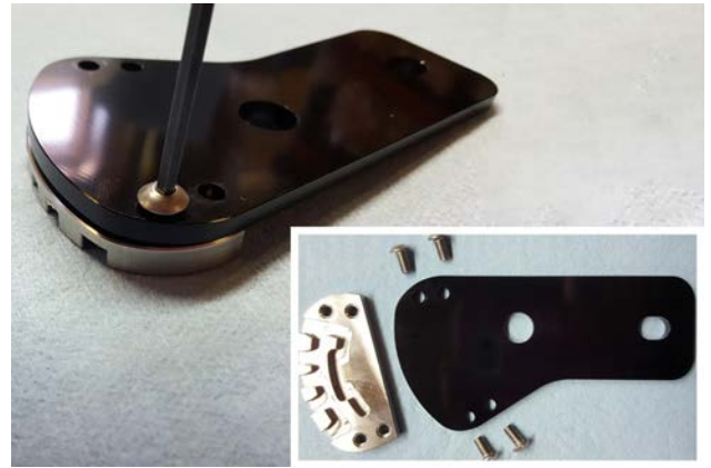
10. Apply loctite to screws (x4) (5) and use them to fasten gate mount (4) to gate plate (3).
