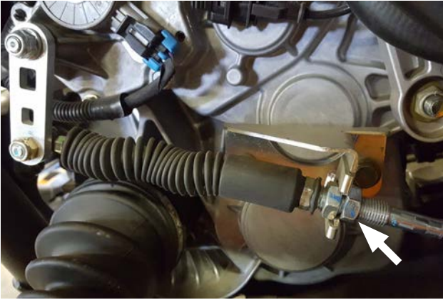
18. Shift through each gear to verify proper function and, if necessary, adjust shifter cable nut for precision.
