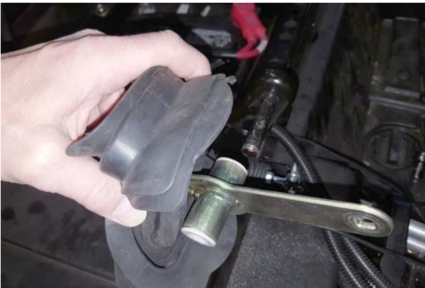
8. Remove shift lever from pivot shaft, taking care not to lose nylon bushings in each end of the bore.
