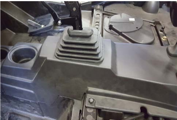
20. Ensure that all components are pulled completely through console then re-install all fasteners (removed step 4) to secure center console.
