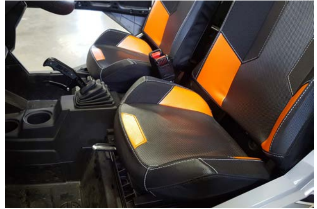
21. Re-install driver and passenger seat into vehicle.
