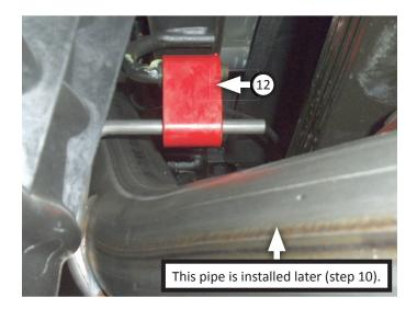
**NOTE:** For 2013-up model year trucks, you must trim 4" from back of inlet pipe. 2011 & 2012 models do not require this modification.
