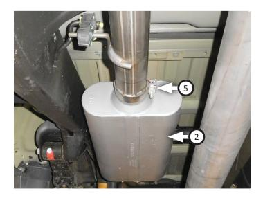
Place rear clamp hanger (4) onto muffler outlet and hang it in isolators. Route tailpipe assembly (3) over rear axle and connect it to muffler, insert wire hanger then tighten clamp hanger for later adjustment.
