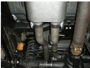
9) Place the front section of the left side tailpipe **#16508S** into the left side muffler outlet and connect the hanger on the pipe to the rubber mount on the vehicle. Tighten the 2 1/2" clamp on the muffler outlet just enough to hold in position.
