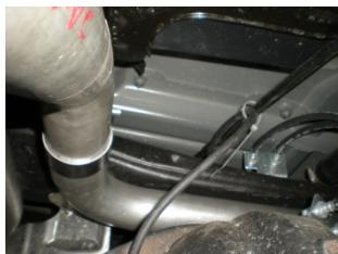
10) Install a provided 2 1/2" clamp onto the slip-fit of left side tailpipe **#16510S**, and then connect to the back of the front section by sliding the two sections together at the slip-fit connection over the rear axle. Place the hanger at the rear of the tailpipe into the rubber mount installed in step 4. Tighten just enough to hold in position.
