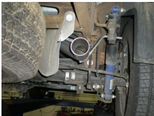
8) Place a provided 2½" clamp onto both muffler outlets, place right side tailpipe **#16758S** into position over the axle and slip into the right side muffler outlet. Connect the hangers on the pipe to the rubber mounts on the vehicle. Tighten the clamp just enough to hold in position.
