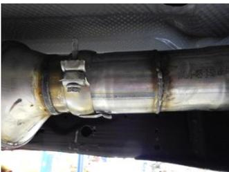
1) Place inlet pipe assembly **#36064S** into position onto the ball connection behind the catalytic converter. Reinstall the clamp onto the ball connection and tighten enough to hold, but still allow for a small amount of adjustment. Connect the hanger on the pipe to the rubber mount on the vehicle.
