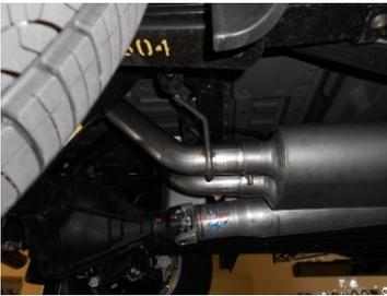
5) Place two of the supplied 2-1/2" clamps over the right and left outlets of the muffler. Place right tailpipe **#86095S** into position over the rear axle, and slide into the right muffler outlet. Connect the two hangers on the pipe to the rubber mounts on the vehicle. Pipe should be approximately 3/4" away from the shock when adjusted.
