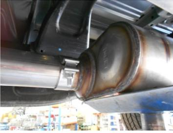
3) Place a supplied 3 1/2" clamp over the inlet of the muffler and then slide the inlet of muffler onto the back of the inlet pipe. Use a stand to support the muffler. Tighten the clamp just enough to hold in position.
