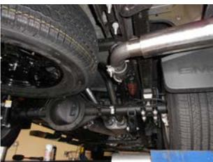
7) Slide the side exit pipes **#26433S** or the rear exit pipes **#26454S** onto the ends of both over axle pipes and place a supplied 2-1/2" clamp onto these slip-fit connections. Tighten just enough to hold in position. Place the two stainless tips **#ST462B** onto the exit pipes and tighten them enough to hold position. Rotate the exit pipes and tips to the desired distance from the body or bumper, so that the angle cut on the tips are in the desired location.
