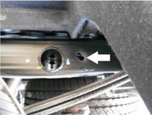
4) Slide rubber hanger **#HA168** onto the end of **226HA**, then using the supplied bolts, washers, nuts and backing plate **#HA226**, mount the assembly to the frame on the left side of the vehicle using the angled oblong hole on the frame rail. *Note: the backing plate #HA226 goes on the inside of the frame between the washers & nut to cover the oblong hole so that the frame hanger won't bend into the oblong holes.*
