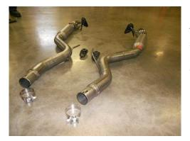
1) Place the new Flowmaster muffler assemblies next to the factory units and swap the front and rear hanger mounts from the stock mufflers to the Flowmaster assemblies. Also, place a provided 2.50" clamp onto the inlet of each assembly. Tighten the clamp just enough to hold in place.
