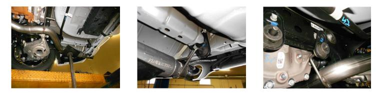
2) Place the right muffler assembly **#815430-405** up into position and slide the inlet completely onto the factory pipe. Support the assembly with a stand and remount the rear hanger mount to the frame, tighten securely. Remount the front hanger to the cross member and tighten securely. Leave the clamp on the inlet loose for now. Repeat this step with muffler assembly **#815430-404** on the left side of the vehicle.
