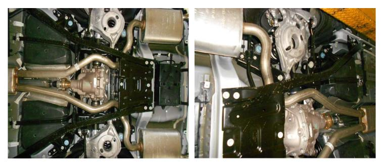
2) On convertible model vehicles, the body braces show in the photos above will need to be removed in order remove the factory system and install the Flowmaster system. Starting at the front of the right side (passenger) brace, loosen the front bolt and then work your way to the rear of the vehicle removing the next eight bolts, lower the brace from the vehicle. Repeat this step on the left side of the vehicle with the six bolts on that side.
