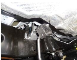
2) Place the factory hanger mounts back into position and secure them to the frame using the factory bolts, tighten securely.
