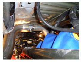
1) Place the supplied clamp onto the inlet of the new Flowmaster muffler, then place the muffler up into position and slide the inlet onto the factory over-axle pipe. Line up the notch in the inlet pipe with the tab on the over-axle pipe, slide on completely. Support the muffler with a stand.
