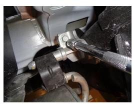
4) Then, use a 13MM socket wrench to remove the upper bolt on each mount. Once both hangers are un-fastened, carefully lower the stand and with the help of an assistant slide the muffler off of the inlet pipe and remove from the vehicle.
