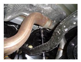
2) Using a 15mm socket, loosen the clamp at the muffler inlet connection above the rear axle.
