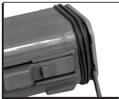
Figure 5 Disassembling the Male Housing.
