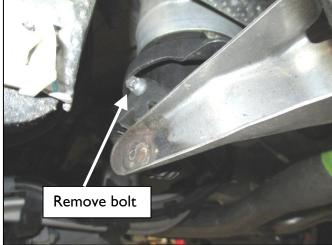
3. Remove the rubber hangers and the weight from the stock mufflers. (SAVE THE MOUNT, MOUNTING BOLT AND RUBBER HANGERS FOR INSTALLATION OF THE DINAN MUFFLER!)
