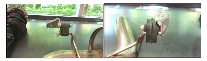
I3. Slide the included muffler tube clamp over the exhaust tube. Install muffler with the clamp evenly over the exhaust tube and muffler tube as shown, and gently snug the clamp bolts. Then finish hanging the muffler using the stock left and right hanger nuts.
