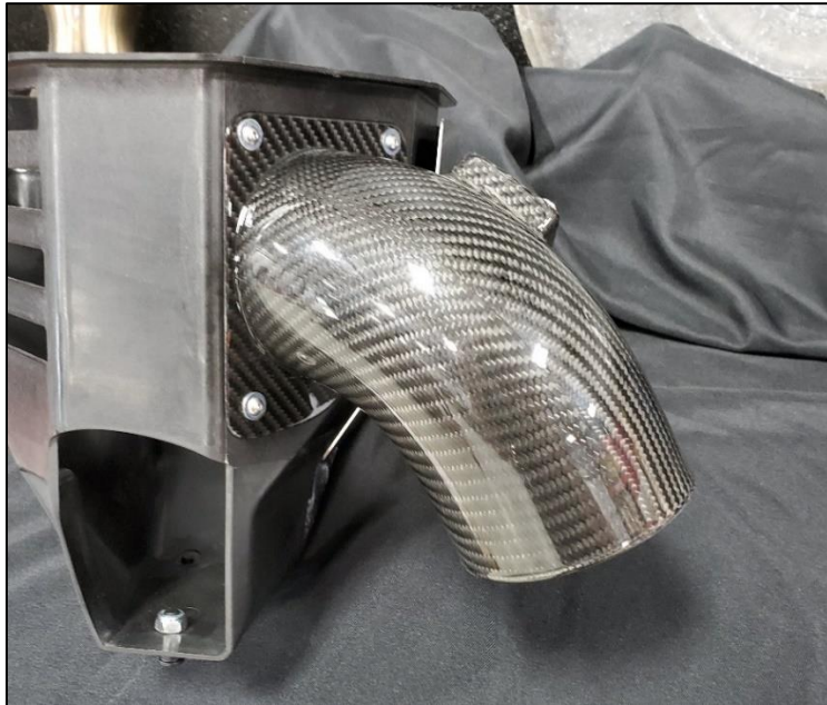
Figure 4: Intake Tube + Lower Box Assembly
