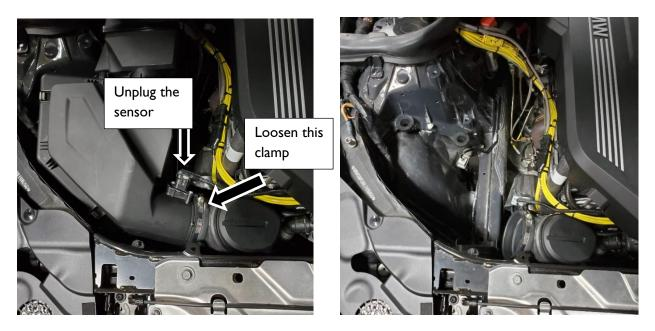
3) Remove the air temperature sensor from the stock intake and carefully place it to the side.
