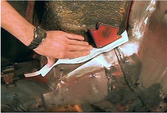
Figure 4 - Inner Wheelwell Front Template
