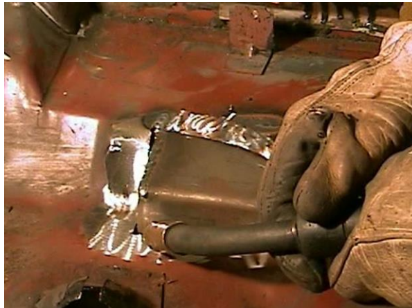
Figure 10 - Welding the Leaf Spring Pocket
