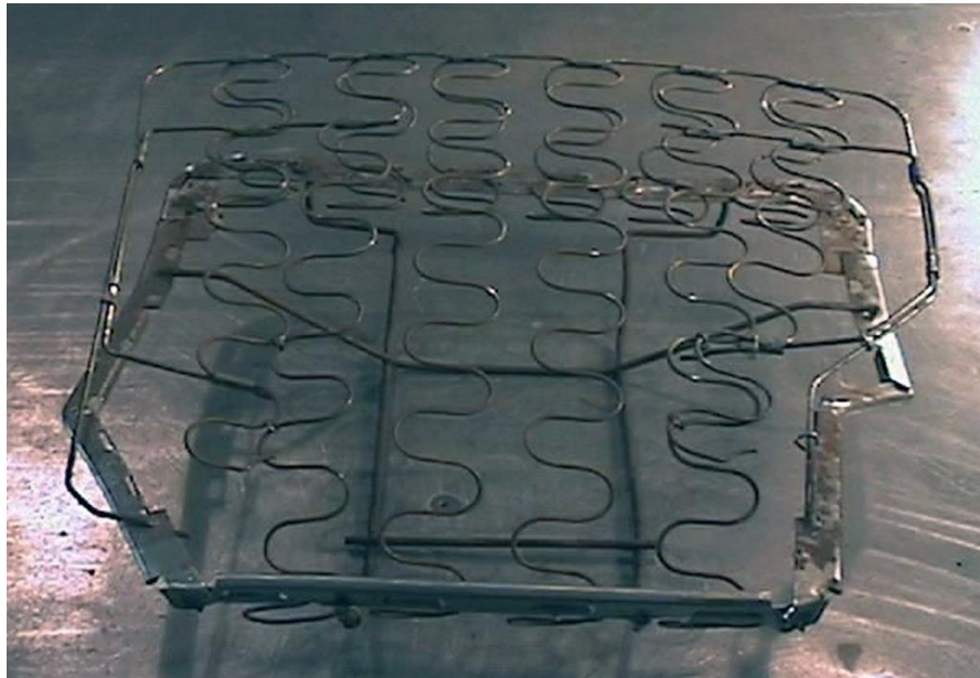
Figure 2 - Narrowed Rear Seat Frame
