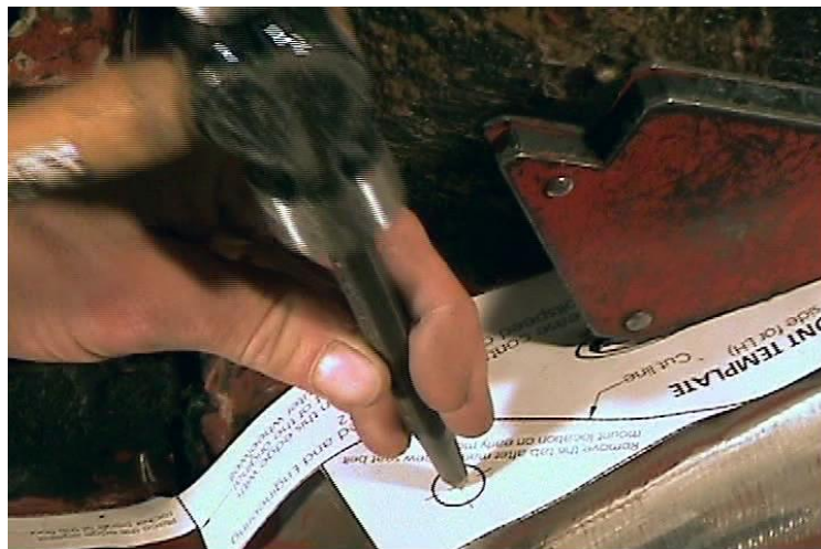
Figure 3 - Inner Wheelwell Front Template with Tab
