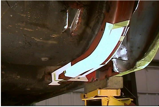
Figure 3 - Inboard Frame Rail Template
