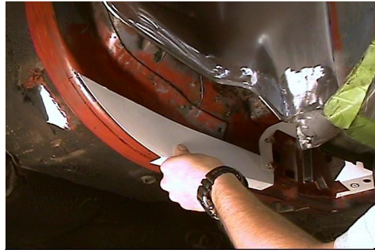
Figure 4 - Outboard Frame Rail Template
