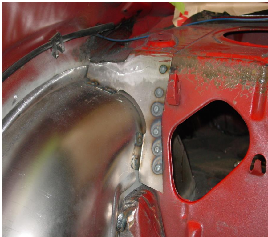
Figure 22 - Seat Back Bracket Installed
