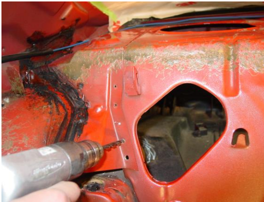
Figure 1 - Seat Support Cut Line
