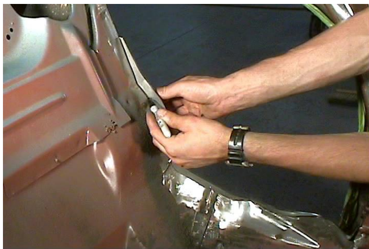
Figure 13 - Marking Front Template to Floor Pan Profile
