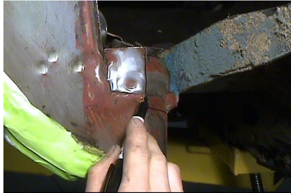
Figure 7 - Marking Tab for Removal
