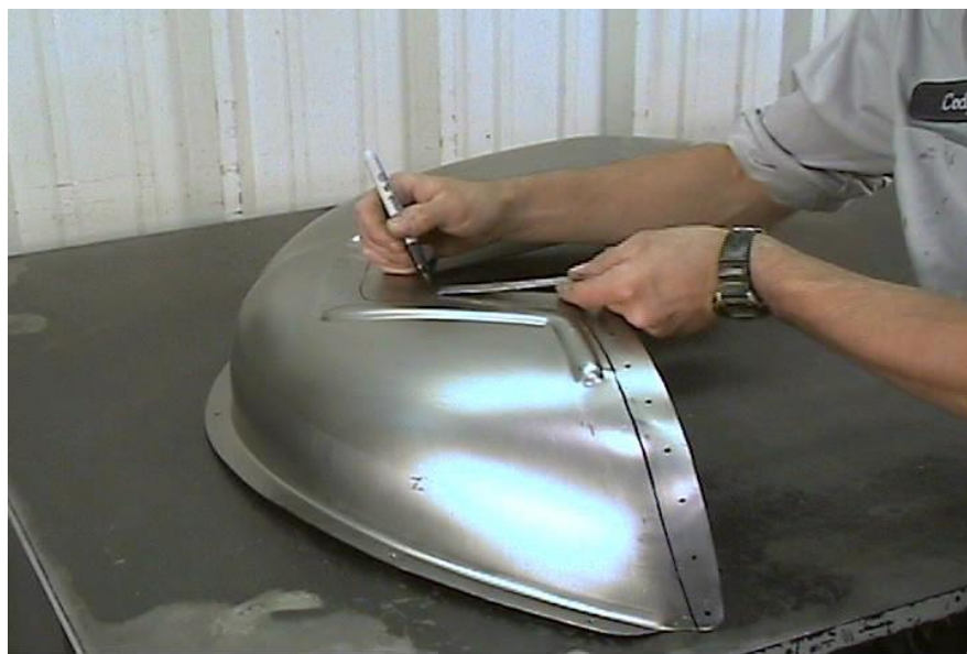
Figure 16 - Mark Tub Mounting Surfaces
