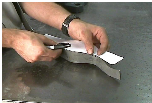
Figure 11 - Front Template Bend Profile
