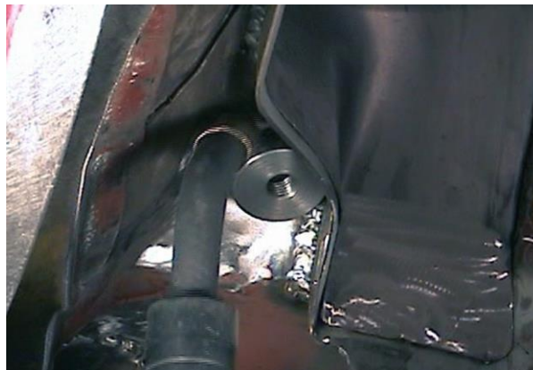
Figure 4 - Weld Seat Belt Mount
