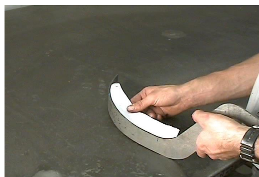
Figure 12 - Rear Template Bend Profile
