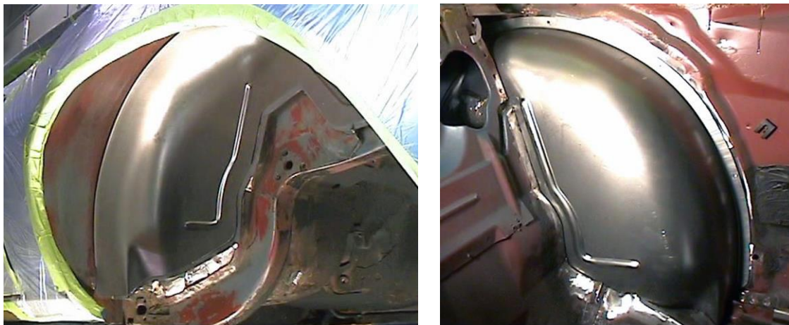
Figure 15 - Test Fit Detroit Speed Mini-Tub
