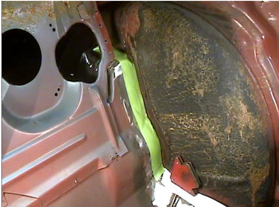
Figure 6 - Cut Line Extension Using 2" Tape
