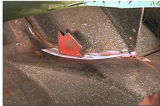
Figure 5 - Inner Wheelwell Rear Template
