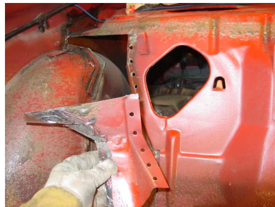
Figure 2 - Seat Support Removed
