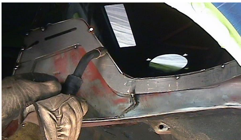
Figure 14 - Tack Weld Tub Flanges
