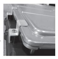
top going through the slot in the stock ECM bracket. Reinstall the 13mm bolt while making sure the Pulsar Mounting bracket is level with the stock bracket. (see picture below).
