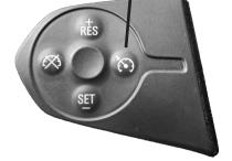
Either turn off Cruise Control or push down on the brake to deactivate High Idle.
