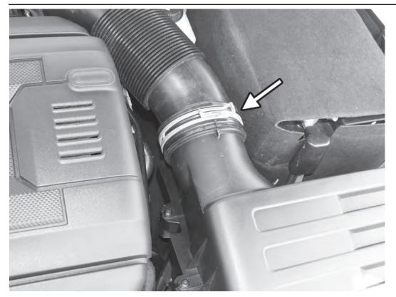
15) Reinstall the stock intake hose, connecting the spring clamp back to the airbox or intake on the car.
