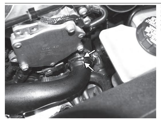
3) With a paint marker or grease pen, mark the orientation of the compressor outlet hose to the compressor outlet pipe on the side of the engine. Be sure to mark both sides. 4) Loosen the two 7mm hose clamps from the compressor outlet hose.
