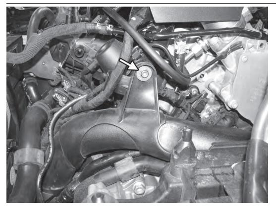
5) Remove the T30 screw from the side of the compressor outlet pipe. Maneuver the pipe slightly out of the way to remove the compressor outlet hose.
