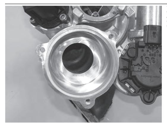
7) Remove the stock turbo muffler from the car. Be sure to remove the o-ring that seals the muffler to the turbo. Do not drop the o-ring in the turbocharger inlet. 8) Loosely place the large supplied APR seal inside the housing of the stock turbo muffler. A small amount of silicone o-ring grease can be used to hold the APR seal inside the stock turbo muffler housing.
