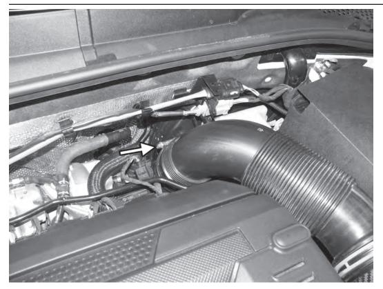
1) Loosen the hose clamp that connects the intake hose to the inlet of the turbocharger. 2) Remove the the spring clamp from the front of the intake hose, and remove the intake hose from the car. Take care not to drop anything inside the turbocharger inlet.
