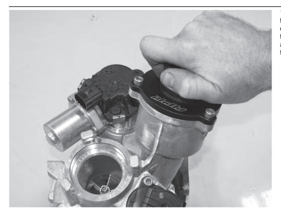
11) Firmly tighten the center section to the outer ring of the APR muffler delete by hand. The center section should compress the APR seal against the bottom of the stock muffler housing. 12) Reinstall the compressor outlet hose to the APR muffler delete and the compressor outlet pipe. Be sure to line up the marks previously made on the compressor inlet hose.
