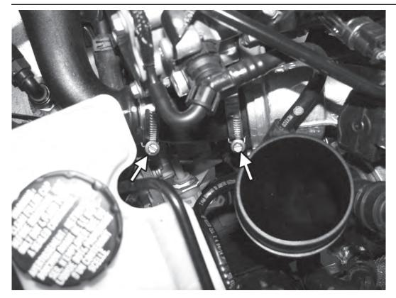
13) Tighten the two 7mm hose clamps on the compressor outlet hose.
